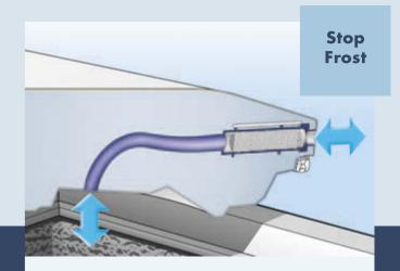
**StopFrost** prevents a vacuum from building up, ensuring the lid opens easily. Frosting over of the freezer and frozen food is reduced, which limits the number of times you need to defrost the freezer.
