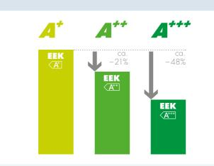
In the best A+++ energy efficiency class, the appliances are approximately 48 % more energy efficient than the top limit of class A+.
