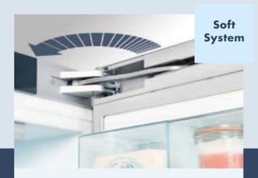
The integrated **SoftSystem** mechanism cushions door closure even when the door shelves are fully stocked; it ensures gentle closing and prevents bottles, jars and packets or food from falling out of the door. The door closes automatically from an opening angle of about 35°. Furthermore, the opening angle of the doors on all BluPerformance models is restricted to 115° to prevent damage to adjacent furniture and to the doors themselves.
